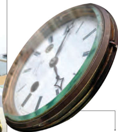
A close up view of the perfect alignment of the "new" bezel to the clock face with the glass that Ellenson cut to fit.
